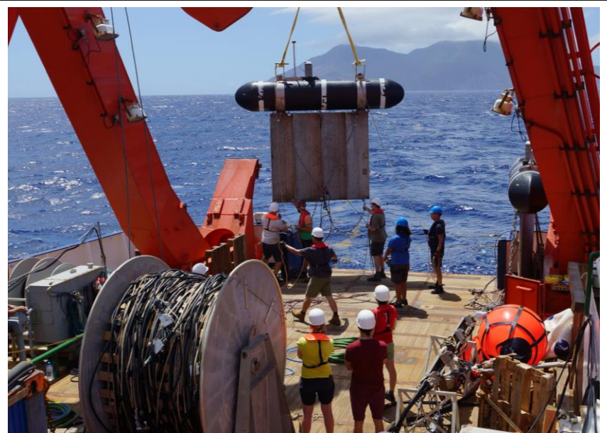
Figure 1: Deployment of the Starboard paravane. Photograph: Stefan Konradowitz.
