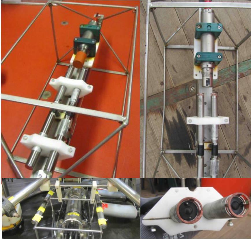
Figure 12 Implementation of two HydroFlash® O 2 optodes at the Cape Verde Ocean Observatory mooring at 120m. Top-left: Measuring cage before the deployment. Bottom-left: CTD calibration setup before the deployment. Top-right and bottom-right: Measuring cage and optode sensor spots after the recovery.
