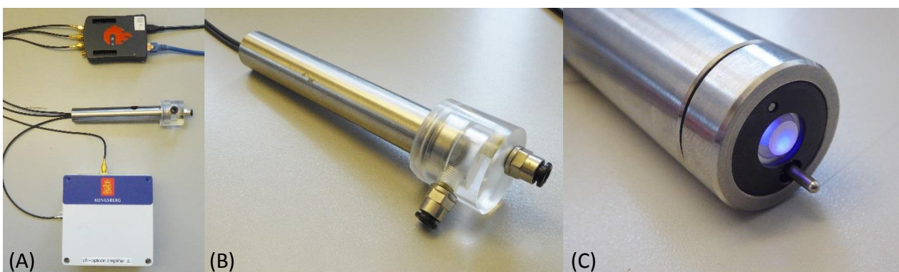
Figure 9 (A) Test setup of the optode prototype incl. function generator and oscilloscope on top, pressure housing with sensing spot in the middle, signal amplifier at bottom. (B) Flow-head at top of the pressure housing. (C) Excited pH sensing spot.
