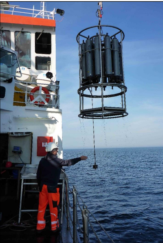
Impressions of cruise AL521. Clockwise from top left: CTD and plankton filtering, fish sampling on board, trawl net coming in, water sampler. Photos: J. Dierking
