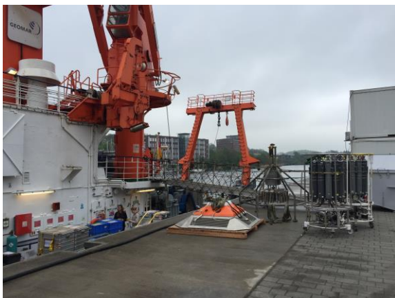
Fig. 1a: Lander, Multicorer and two CTDs still have to be loaded (courtesy of M. Schmidt).
