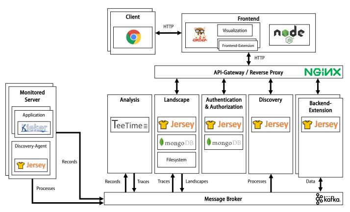
Figure 3: Architectural overview and software stack of the restructured ExplorViz.
