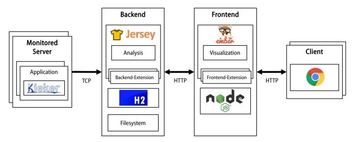
Figure 2: Architectural overview and software stack of the modularized ExplorViz.
