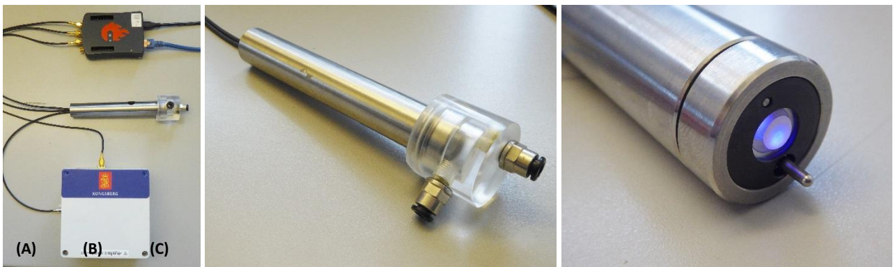
Fig. 8: (A) Test setup of the optode prototype incl. function generator and oscilloscope on top, pressure housing with sensing spot in the middle, signal amplifier at bottom. (B) Flow-head at top of the pressure housing. (C) Excited pH sensing spot (from AtlantOS D6.3).
