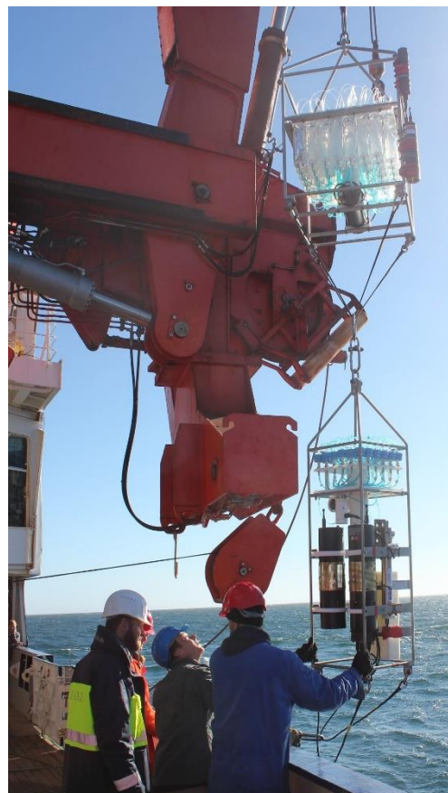
Fig. 3. Concurrent deployment of the RAS-500 water sampler and the PPS particle sampler during POLARSTERN cruise PS 99 in Fram Strait (image: I. Salter, AWI)
