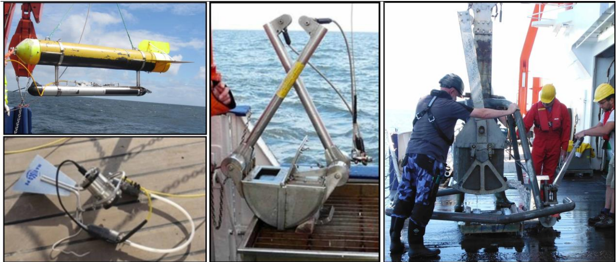
Figure 2: Overview of some of the used methods /from left to right): Sidescan sonar system attached to bouancy element, underwater video camera, HELCOM grab sampler, giant box corer.
