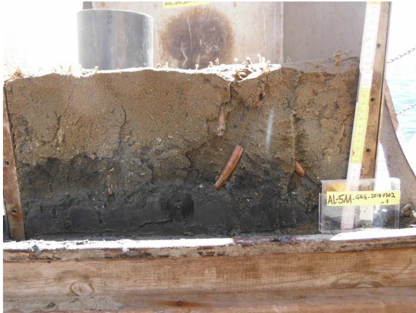
Figure 8: Giant box corer sediment sample AL-511-GKG_20170702_1 from Hever tidal channel (54° 19,904'N 8°14,388'E). Ensis sp. burrows can be observed down to 15cm. Ensis sp. is capable to quickly pull itself back into the sediment.
