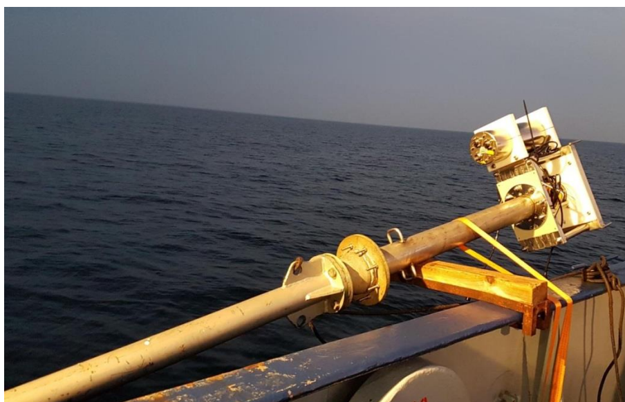
Figure 3: Side pole on the aft deck with the Subbottom Profiler attached.
