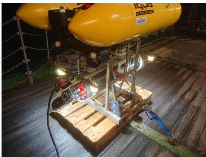
Figure 15: Anton equipped with 4 new LEDs.
