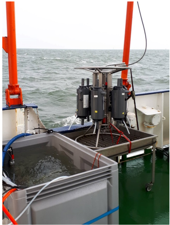
Figure 2. The water tank used for sensor deployments (on the left side) and the Niskin bottles of CTD vertical profiler (on the right side) (photo credit: M. Nehir)
