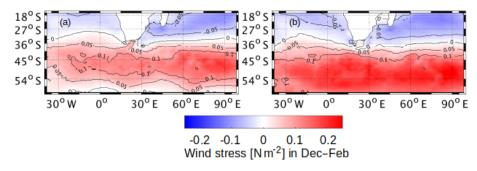
**Figure 3.** Temporal mean of the December–February wind stress ( $Nm^{-2}$ ) for the periods 1964/1965 (a) and 2007/2008 (b) derived from the COREv2 data set. Contours and shading represent the same variable.
