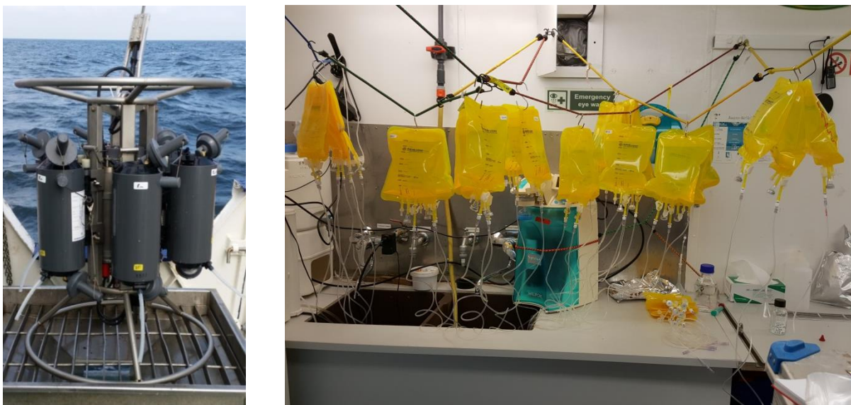
Figure 42: (Left) Mini-Niskin bottle rosette for collecting vertical profile water samples. (Right) Gravity setup for MC extraction from seawater.
