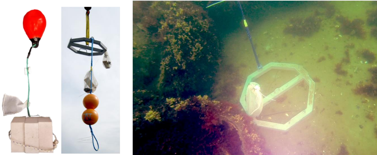
Figure 43: Moorings used for bio-monitoring with blue mussels. (Left) A mooring used for shorter time periods together with lifting body, mussel net and three stones as anchor (6,6 kg each). Two passive samplers are fixed to the rope above the net. (Middle) A mooring used for longer time periods hanging upside down on a ship crane, together with two lifting bodies, a steel anchor (100 kg), two mussel nets with mussels and a piece of wood inside the nets, to allow the mussels to attach themselves. (Right) Mooring on the seafloor, in direct vicinity to two moored mines.
