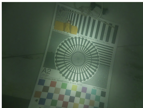
Fig. 7. Calibration board mounted in a test basin, 1.5 m in front of a PlasPi camera.
