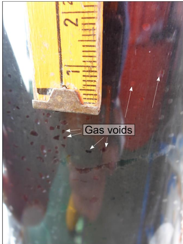
Figure 7: Voids in the sediment cores containing free gas immediately after core recovery (core FL18).
