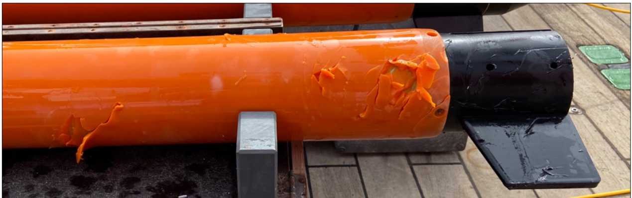
Figure 5.1: Damaged rear tow-fish after a shark attack. The magnetometer is fully functional but the rubber coating was damaged and one fin missing.
