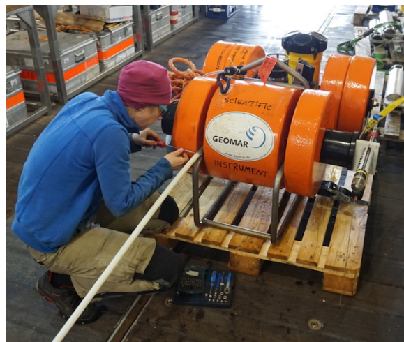
W. Martens disassembling the bottom-lander in the hangar of the Merian (Photo: J. Karstensen)
