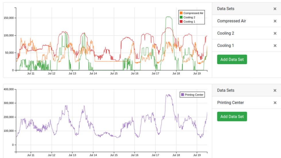
Fig. 5 Screenshot showing the graphical correlation of power consumption using the Titan Control Center
