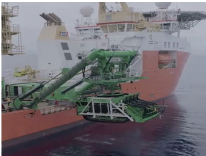
Fig. 7: The scaled prototype of the Mn-nodules collector Patania II during launching operation
