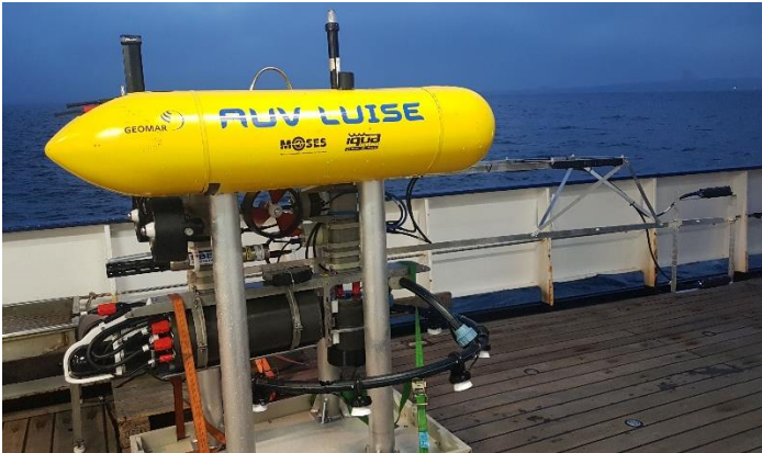
AUV Luise with magnetic 'horn' carrying two magnetic sensors above each other.
