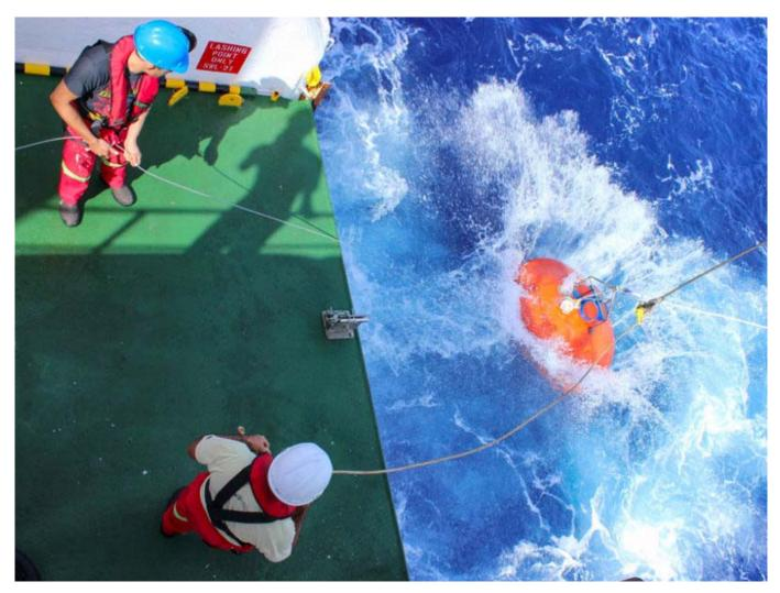
Technicians on board the R/V *Algoa* in 2015 deploy oceanographic instrumentation along the Agulhas System Climate Array to provide long-term observations of the Agulhas Current, a western boundary current of the southwest Indian Ocean. Credit: Jarred Voorneveld By <u>Jordan Van Stavel</u>, Johannes Karstensen, <u>Juliet Hermes</u>, and Jay Pearlman ② 25 August 2020
