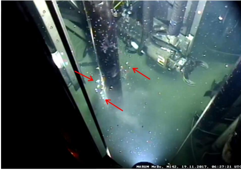
Figure S6 Image taken from the inside of the MARUM MeBo200 drill rig frame when performing operations at Site GeoB22605-1 (MeBo17). The photo was taken on November 19, 2017 when drilling reached a depth of 143.85 mbsf, close to the expected depth of the BSR-1. Free gas bubbles escaped from the borehole (examples indicated by red arrows) and deeper drilling was stopped.
