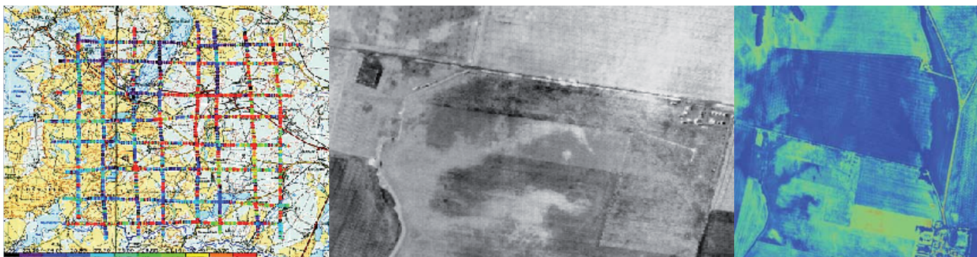
Figure 2. Infrared image (center) of the LITFASS area taken from a Tornado RECCE aircraft of the German airforce and surface temperatures from the HELIPOD (left) which were used to calibrate the infrared images and the calibrated infrared surface temperature from the combination of Tornado and Helipod measurements (right). The reverse “L” shaped central experimental field can be identified in the center picture and in the lower left quadrant of the right picture. Temperatures range from 20 °C (blue) to 55 °C (red).
