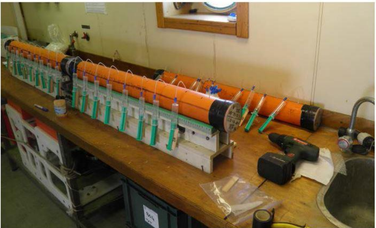
Figure 3: Photograph showing the pore water sampling in the lab on board of RV URANIA. We took samples every 10cm on the first core. In subsequent cores only 3 times per section were sampled.
