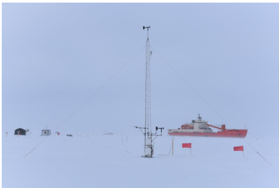
Figure 1. Campbell Scientific gradient meteorological complex in the Ice camp.
