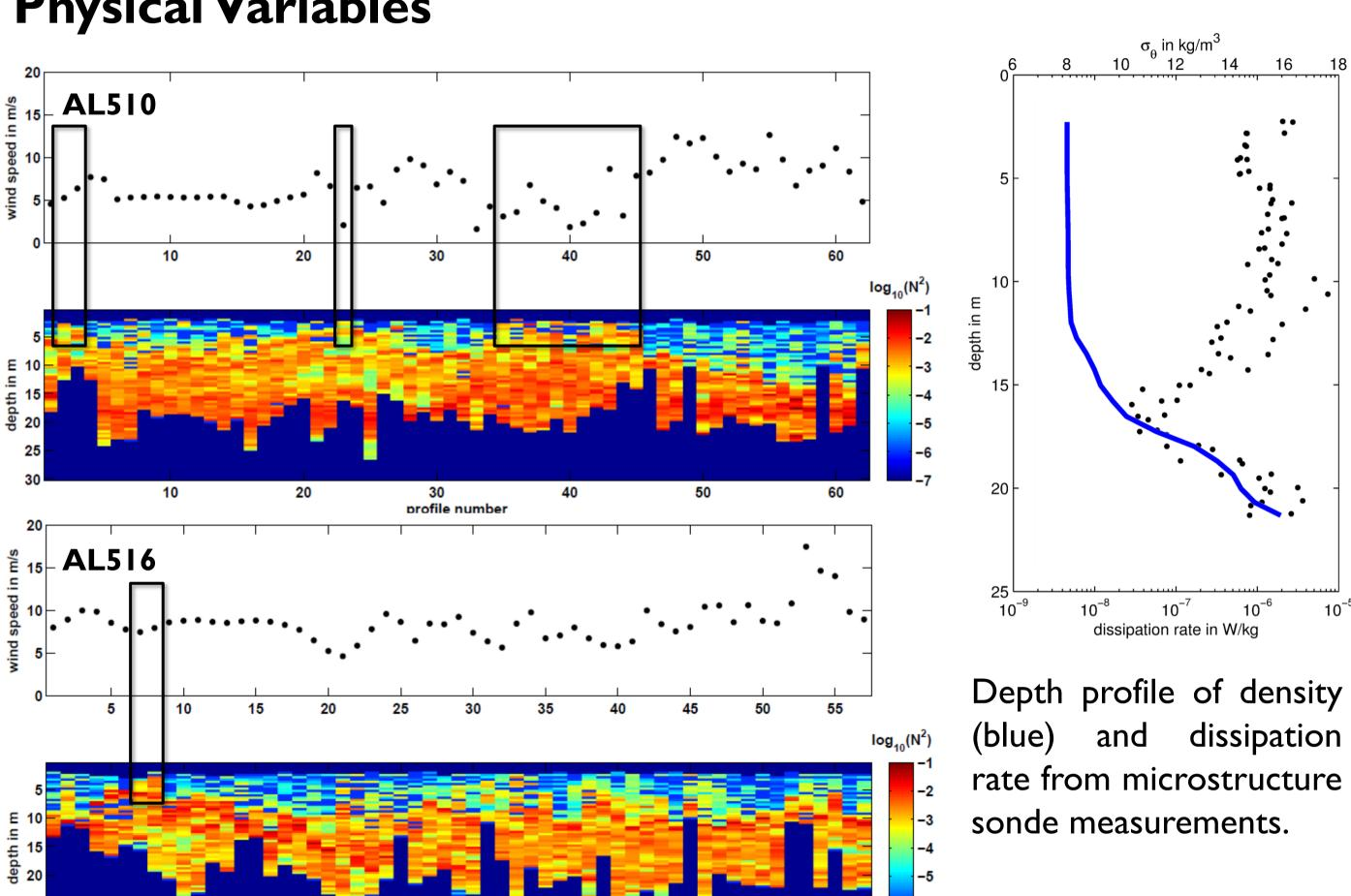
Near surface stratification of the water column was calculated from microstructure sonde measurements deployed from the ship's rubber boat during every station.
