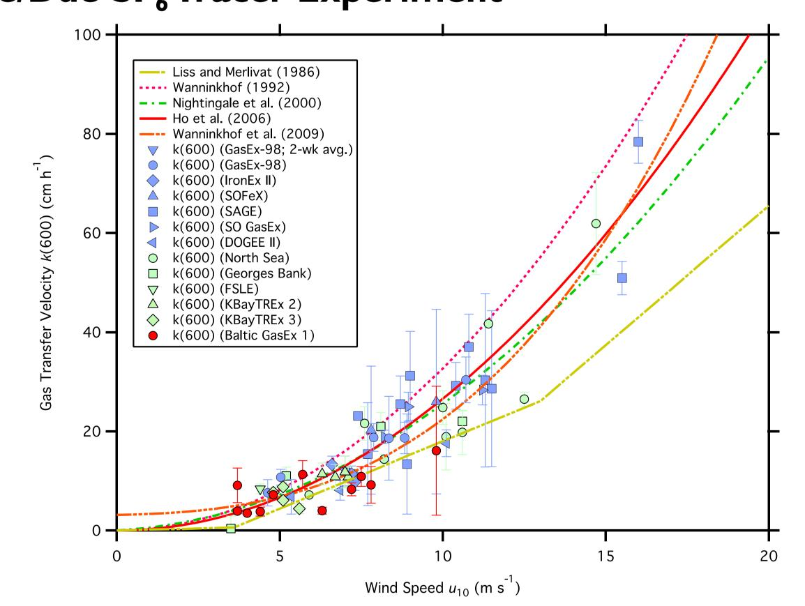
Gas transfer velocities derived from  ${}^{3}\text{He/SF}_{6}$  dual tracer experiment during Baltic GasEx I (AL510) shown along with those from previous experiments, as well as frequently used wind speed/gas exchange parameterizations for the coastal and open ocean.
