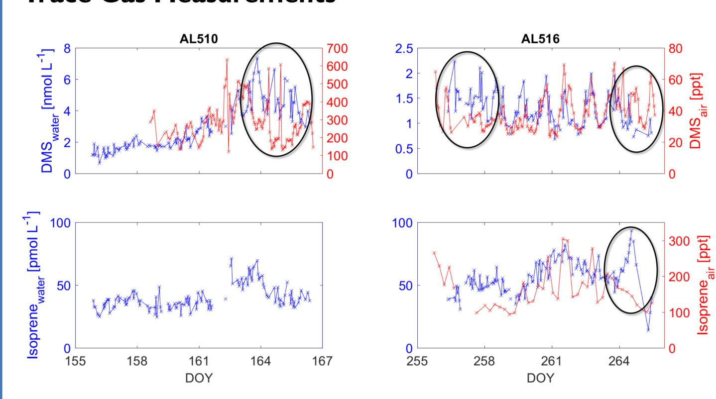
DMS and isoprene air-sea concentration gradients and DMS eddy covariance fluxes were measured with atmospheric pressure chemical ionization mass spectrometry (AP-CIMS, air fluxes) and gas chromatography-mass spectrometry (GC-MS, water).
