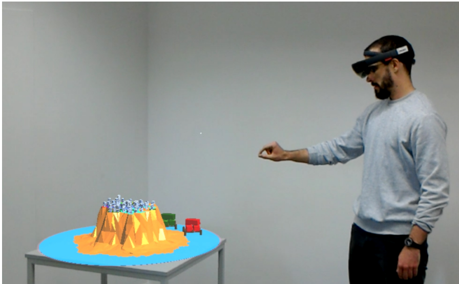
Figure 4.3. AR Visualization of IslandViz [Schreiber et al. 2019]. An "Air-Tap" gesture can be performed to select a bundle.
