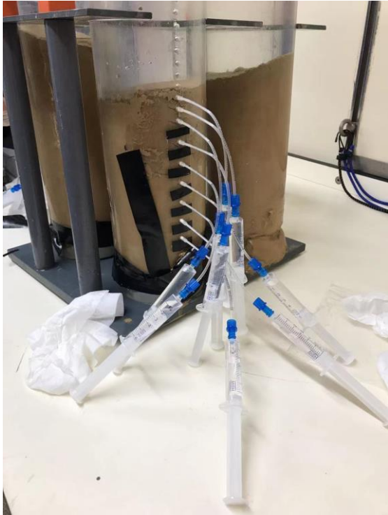
Fig. 2: Porewater extraction from sediment core obtained under Rainbow plume (ca. 2300 m). Photo Zhouling Zhang
