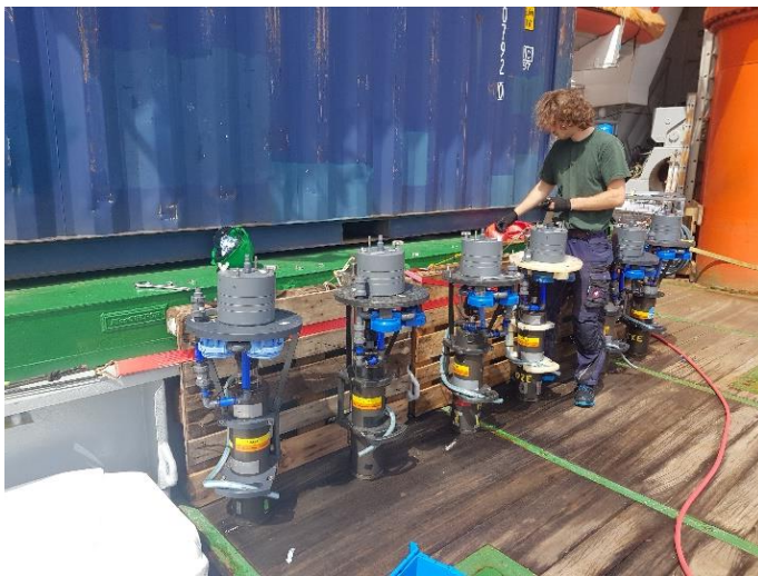
Fig. 1: In situ pumps on deck after deployment at ca. 2100 m. Photo EA
