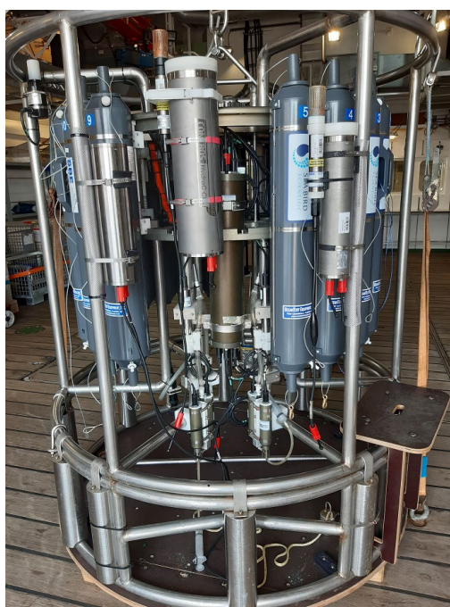
Figure 5.2.1 Deploying the CTD-device of RV M.S. Merian. Water sampler (21x10 L Niskin ) rosette includes SBE9plus-CTD, O 2 , turbidity (Wet Labs), methane (Contros), CO 2 (Contros), nitrate (SBE) and PAR sensors.
