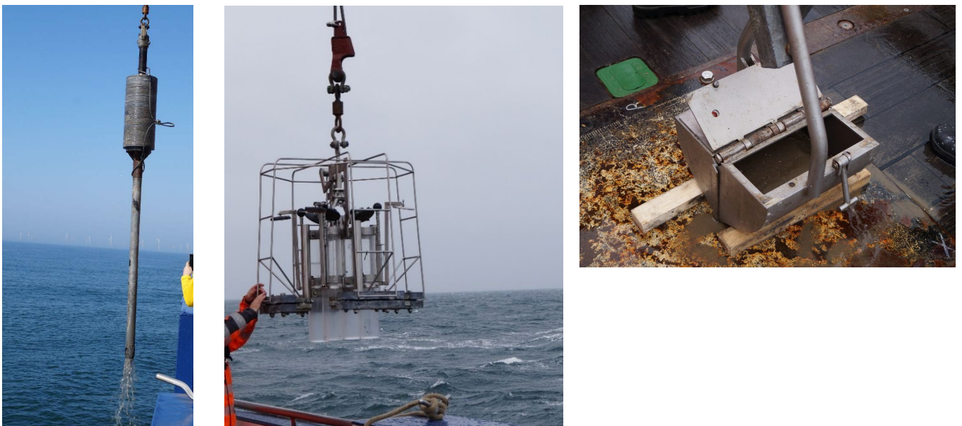
Figure 5.3.1. Deployment of gravity corer (left), Mini Multi corer (middle) and Van-Veen Grab (right)
