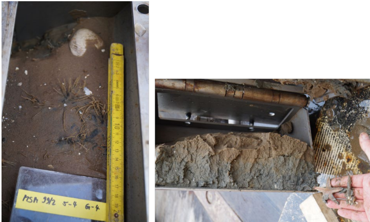
Figure 5.4.1. Left: seafloor surface of grab sample 5-4 G4 that contains brown, massive fine sand Lanice conchilega tube worm and single bivalve shells of Laevicardium crass , Scrobicularia plana and Donax vittatus (in the upper right of the picture); Right: Profile of grab sample 10-1 G7 with Lanice conchilega and a Astropecten jonstoni . Weak redox horizon in the lower part.
