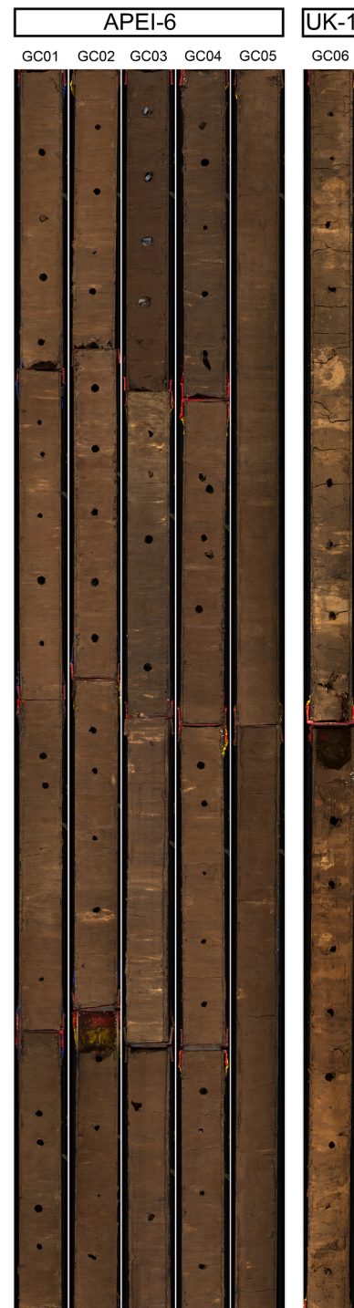
Fig. 4. Photographs of sectioned gravity cores from APEI-6 (GC01-05) and UK1. The image is cropped to the length of the shortest core (GC06). For scale, the width of each core is 70 mm.
