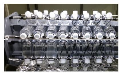
Our phytoplankton communities where exposed to future Ocean Acidification for about 50 generations and kept in suspension by constant rotation on a plankton wheel. The plankton wheel avoids sedimentation of the cells at the bottom of the small bottles which would lead to very unnatural conditions.
