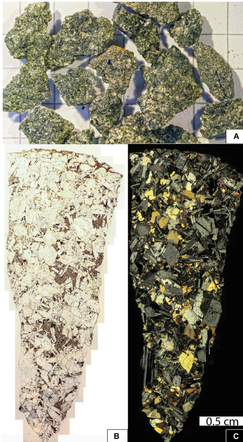
FIGURE 2 | (A) Recovered fresh gabbroic rock fragments. Squares in the background are 1 cm. Thin section of one gabbro fragment in (B) plane-polarized light and (C) cross-polarized light.
