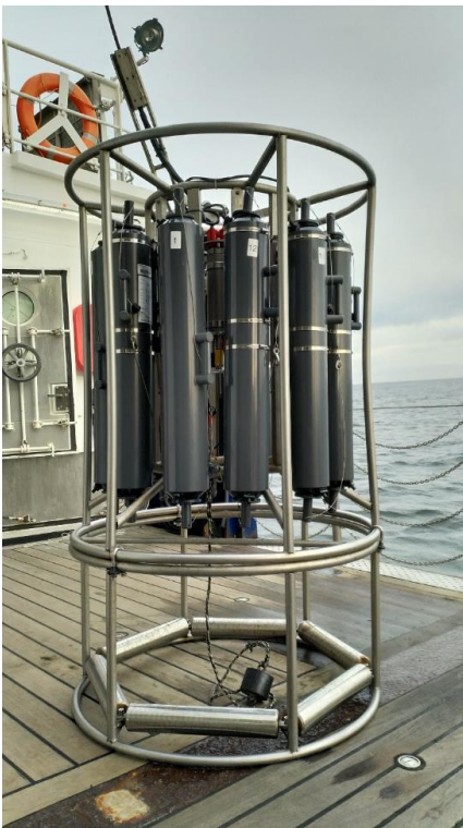
Fig. 5.4.1: The ship's CTD used for most of the CTD surveys.
