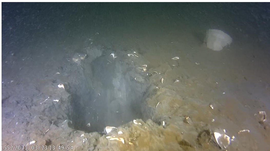
Figure 4.8 Gravity corer hole seen in video profile after sampling
