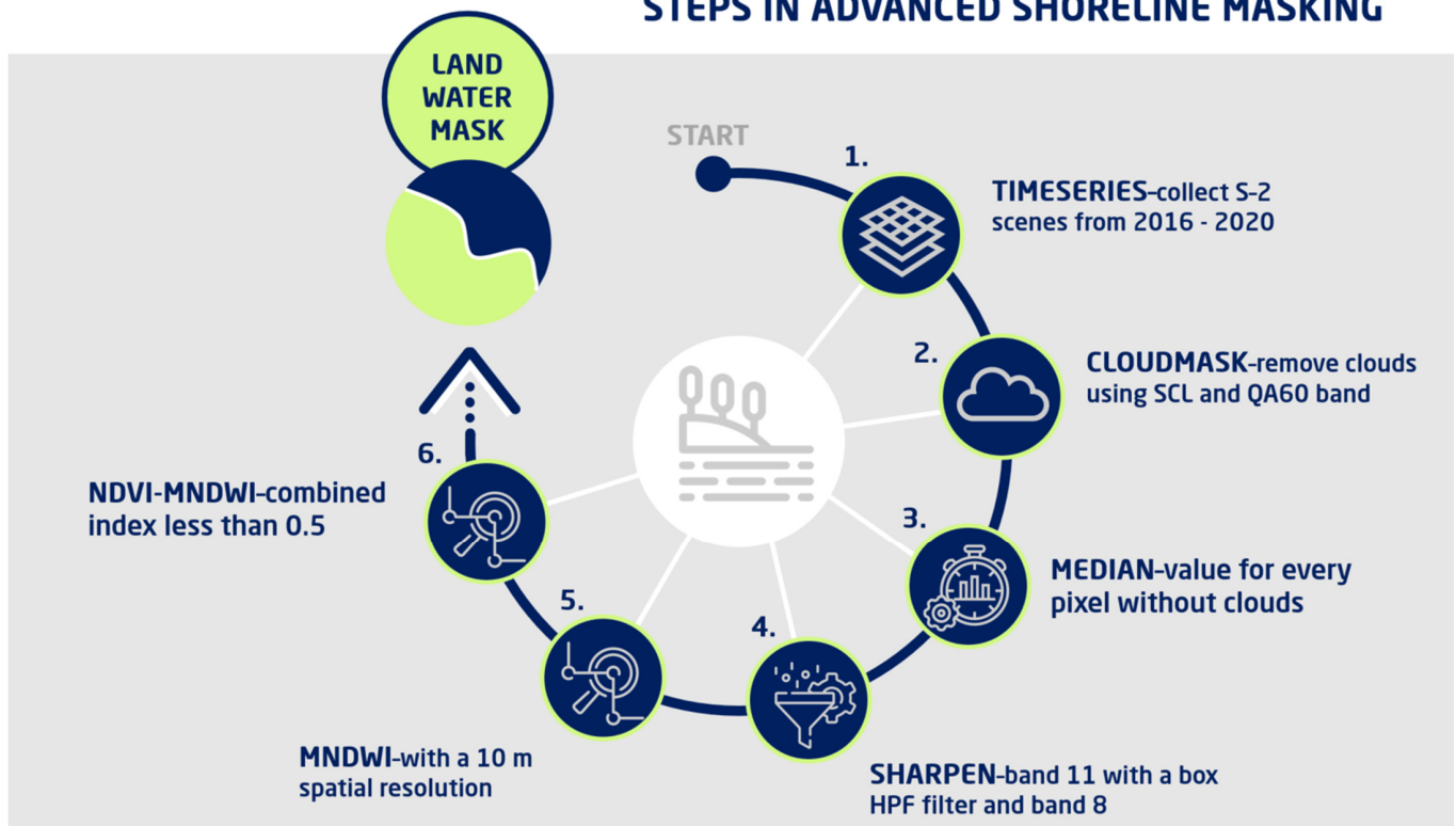
Figure 3. The six steps of the land-water mask creation with preservation of the sandy beach area.
