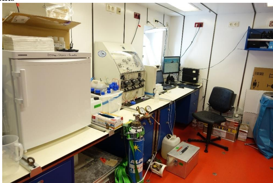
Fig. 12.8 Typical nutrient measurement setup with SEAL-Analytical-Quattro39 Segmented flow analyser on ship
