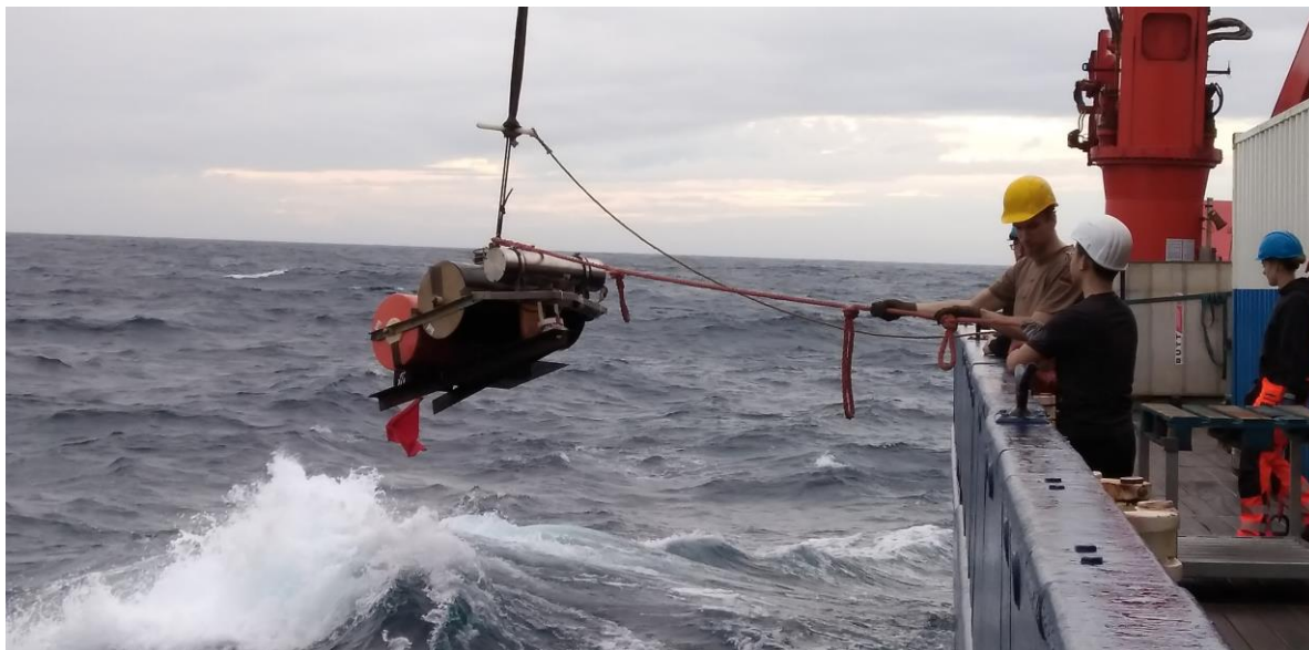
Fig. 12.1 Deployment of a short-period Ocean-Bottom-Seismometer (OBS) (photo: Helene Hilbert)
