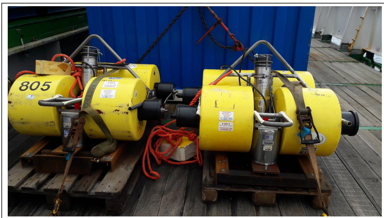
Fig. 12.2 Broad-band Ocean-Bottom-Seismometer (OBS) on deck of RV METEOR
