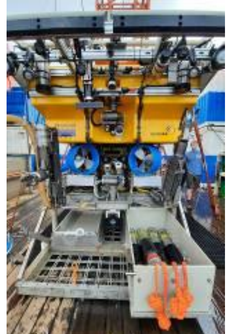
Fig. 5.15 ROV with 4 transponders in its portside drawer.
