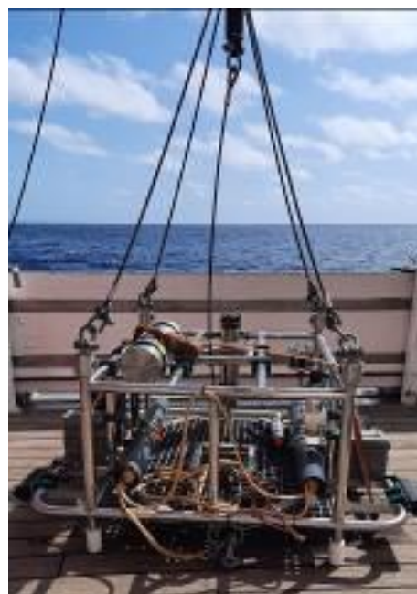
Fig. 5.12 Recovery frame used to retrieve tripods
