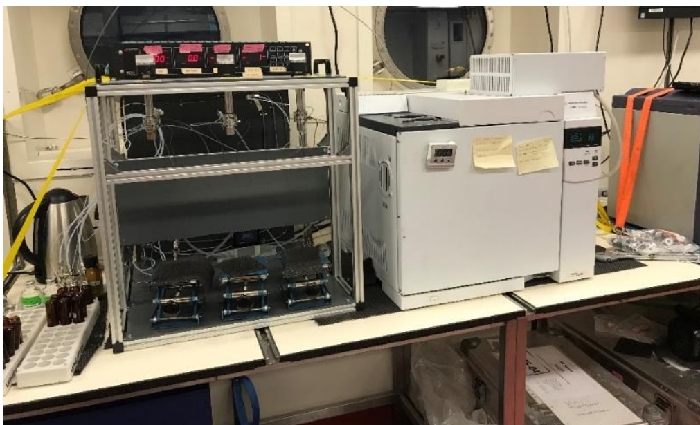
Figure 5.60: System set-up on board. P&T-System (left) and GC-FPD (right) used for DMS measurements.
