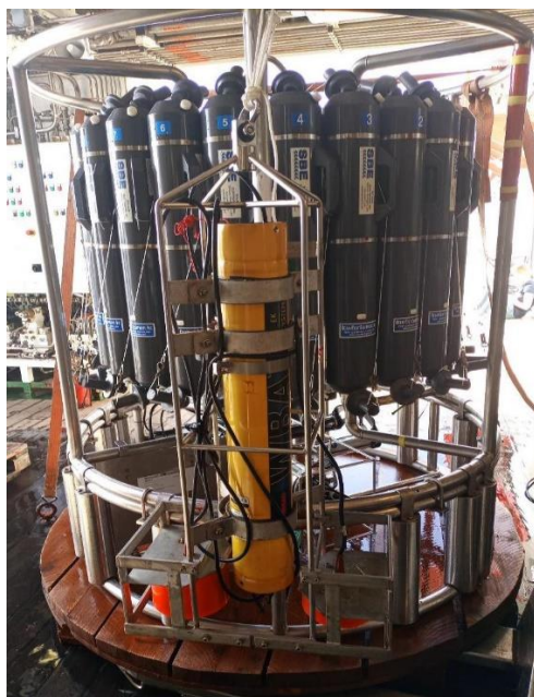
Figure 5.1: WBAT mounted vertically on the CTD rosette.
