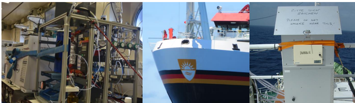
Figure 5.26: left: Purge and trap GC/MS–system (J. Karnatz) for the measurements of dissolved and atmospheric halogenated hydrocarbons, middle: intake line for the air sampling of volatiles in stainless steel canisters with a metal bellows pump, right: Norwich-sampler for the collection of size segregated aerosols.
