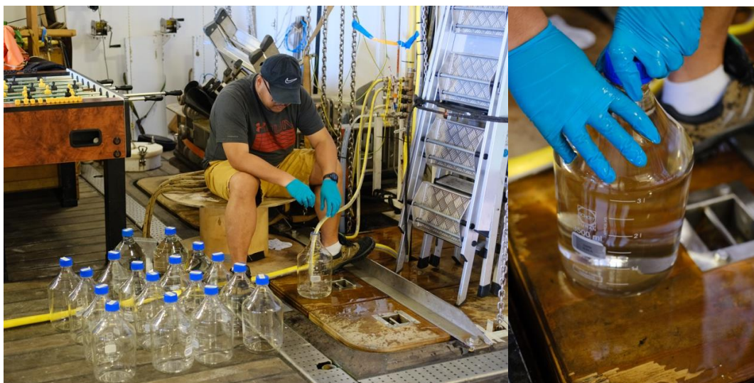
Figure 5.9: Collection of seawater samples in 3.5 L Duran glass bottles for the 48-hour incubation experiment.
