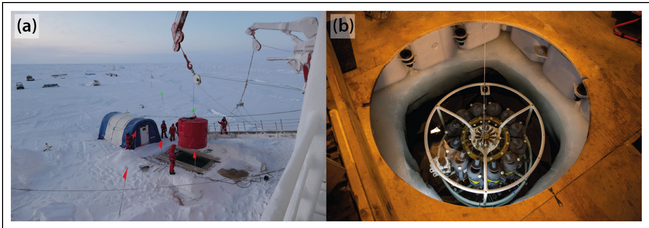
Figure 6. Selected images of installations during operation. Conductivity-temperature profiling through depth (CTD)/rosette with red shelter during operation at the Polarstern -hydrohole and the tent used to protect the hydrohole outside hours of operation (a); CTD/rosette in Ocean City during deployment in the hydrohole (b). Photo credits are Janin Schaffer (a) and Esther Horvath (b). DOI: https://doi.org/10.1525/elementa.2021.00062.f6
