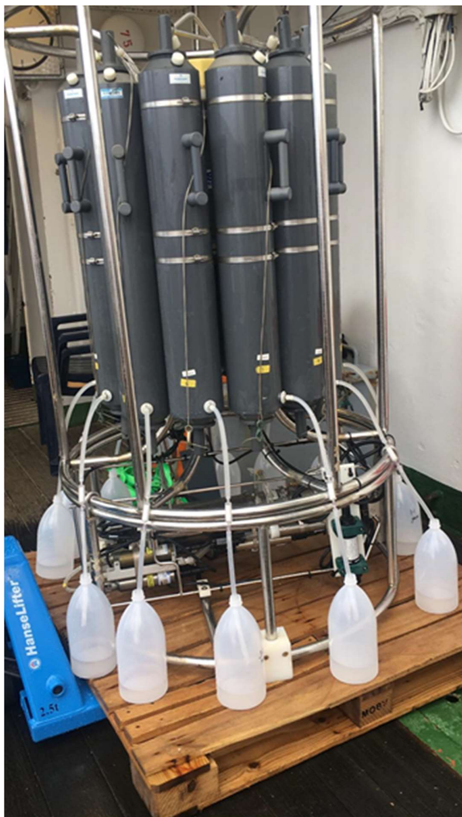
Figure 6: Set up for eDNA filtration. Between the Niskin and the 2L bottle there is a sterivex filter for water filtration.
