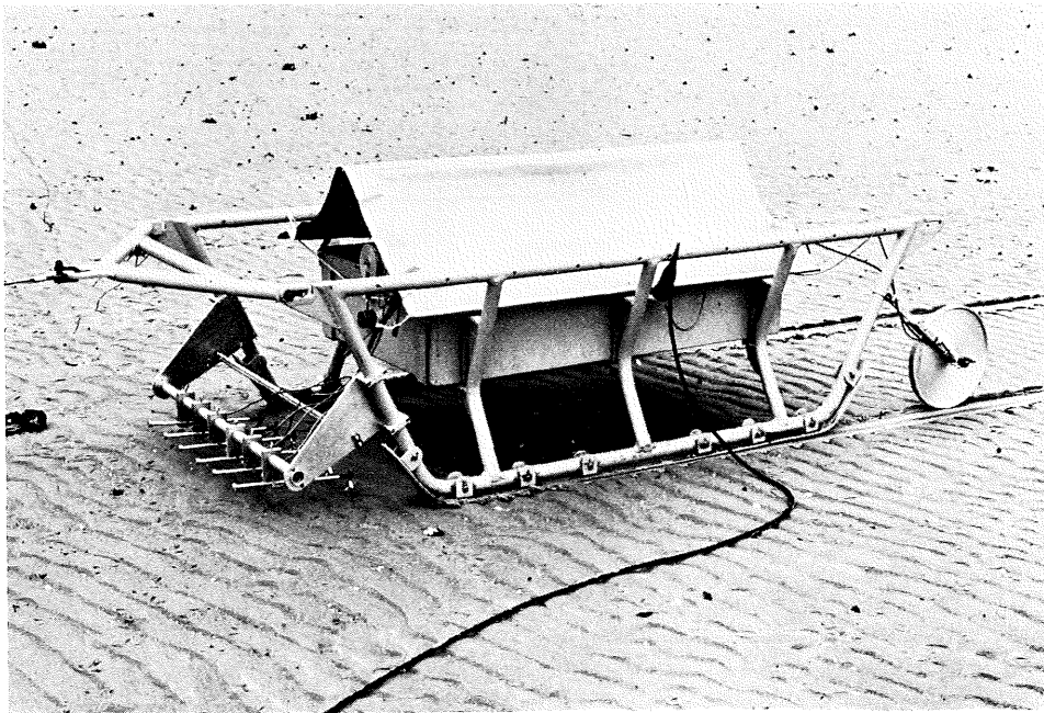
Fig. 2 The ripple profiling sledge with sensors
