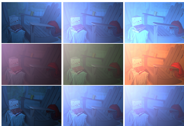
Figure 7. Simulated images vary significantly with different settings of lighting conditions (first row), attenuation parameters (second row), and g in H-G phase function (third row).
