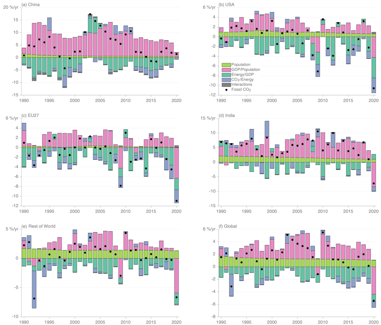
Figure 14. Kaya decomposition of the main drivers of fossil CO 2 emissions, considering population, GDP per person, energy per GDP, and CO 2 emissions per energy use, for China (a), USA (b), EU27 (c), India (d), the rest of the world (e), and the world (f). Black dots are the annual fossil CO 2 emissions growth rate, coloured bars are the contributions from the different drivers. A general trend is that population and GDP growth put upward pressure on emissions, while energy per GDP and more recently CO 2 emissions per energy put downward pressure on emissions. The changes during 2020 led to a stark contrast to previous years, with different drivers in each region.
