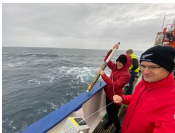
Anne-Sophie Fortin and Jörg Fröhle launching the last uCTD on RV Meteor M184 (Photo: P. Henning)
