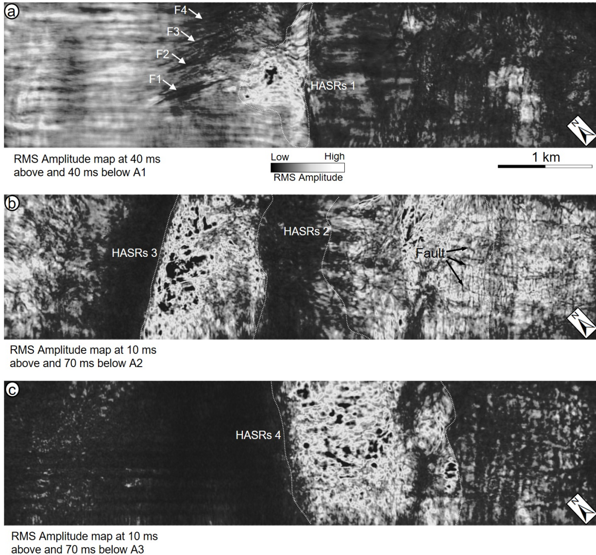
Figure 9. (a) A root mean square (RMS) amplitude map, extracted from 40 ms above to 40 ms below the A1 horizon in the Omake 3D seismic dataset, highlighting the location and distribution of the anomalous reflections characterizing HASRs 1. Dark sub-parallel lines observed to the north of HASRs 1 represent faults: F1-F4. (b) A RMS amplitude map, extracted from 10 ms above to 70 ms below the A2 horizon, highlighting the distribution of anomalous reflections characterizing HASRs 3 and HASRs 2. Dark striping highlight multiple faults that
