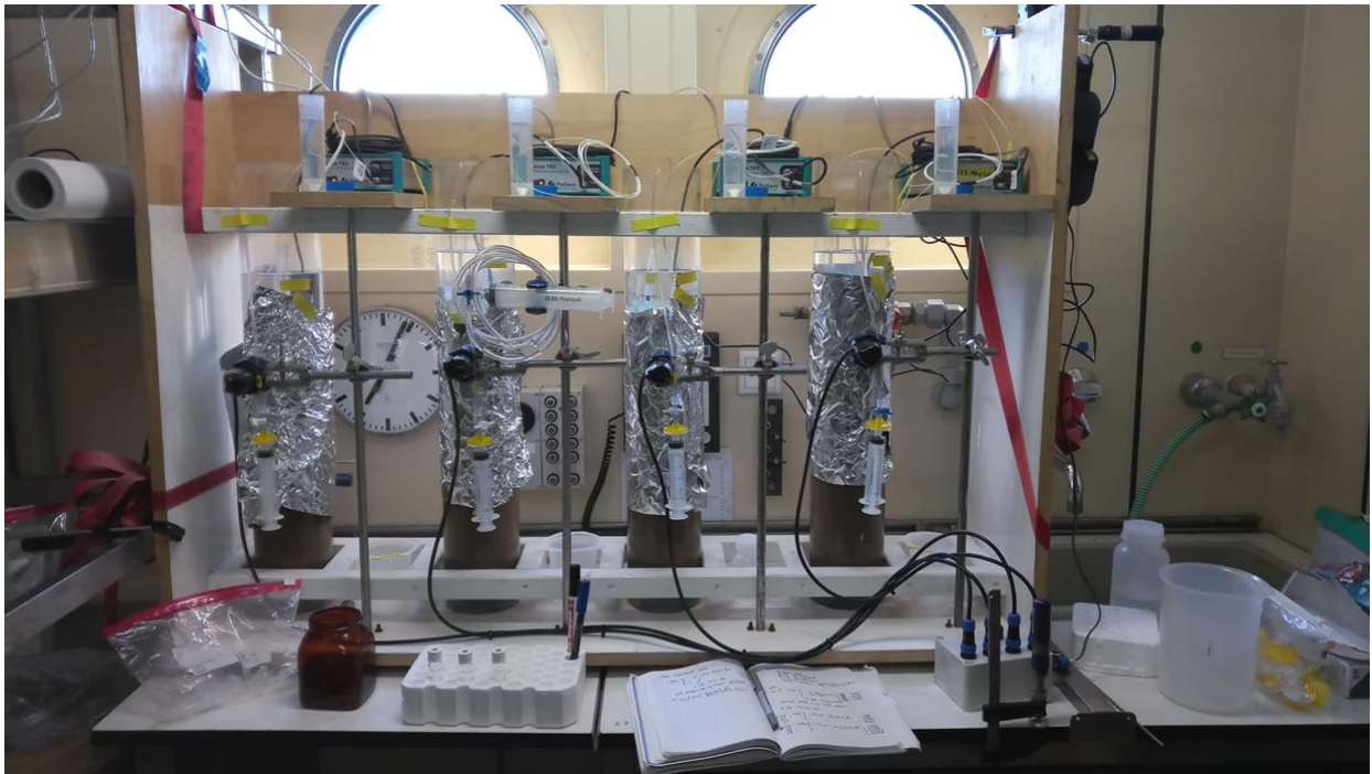
Figure 5.3.5.1: Photo of the whole-core incubation setup in the temperature-controlled lab of RV ALKOR. (Photo: C. Nantke)
