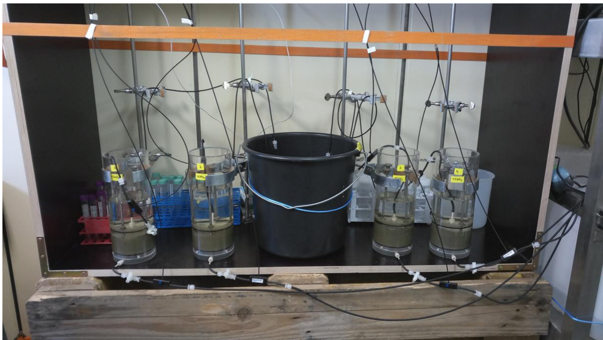
Figure 5.3.4.2: Photo of the FTR incubation setup in the temperature-controlled lab of RV ALKOR. (Photo: C. Nantke)
