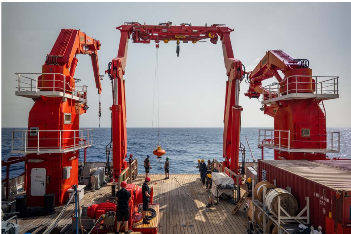
Fig. 1: Mooring deployment of the Cape Verde Ocean Observatory. The top element of the mooring is already in the water. Here, the ADCP (acoustic Doppler current profiler) is just to be deployed, finally being located 300m below the surface (Photo: David Menzel).
