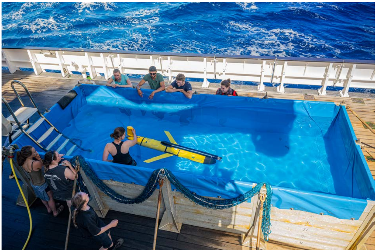
Fig. 4: Test of the autonomous glider in the pool aboard RV Sonne. The glider (yellow) is equipped with several hydrographic sensors and a microstructure probe, which is the black piggyback instrument on top of the glider (Photo: David Menzel).
