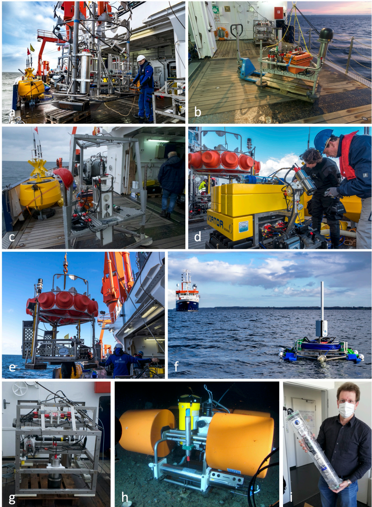
Fig. 5.1.2 The ARCHES underwater network consists of the following mobile and stationary sensing platforms. BIGO-Lander, b. CRAWLER SIM, c., FLUX Lander, d. VIATOR, e. MANSIO, f. WLAN-Katamaran (in the background the RV ALKOR is visible), g, towed camera and sensor system OFOS, h, SLM Lander, i. acoustic recorder. Photos: Submaris, Flögel, Sommer, Walter, Wenzhöfer.
