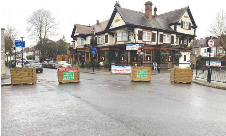
Figure 4.6: West Ealing South LTN21 – Modal Filters and Planter Boxes Aimed at Traffic Restriction
