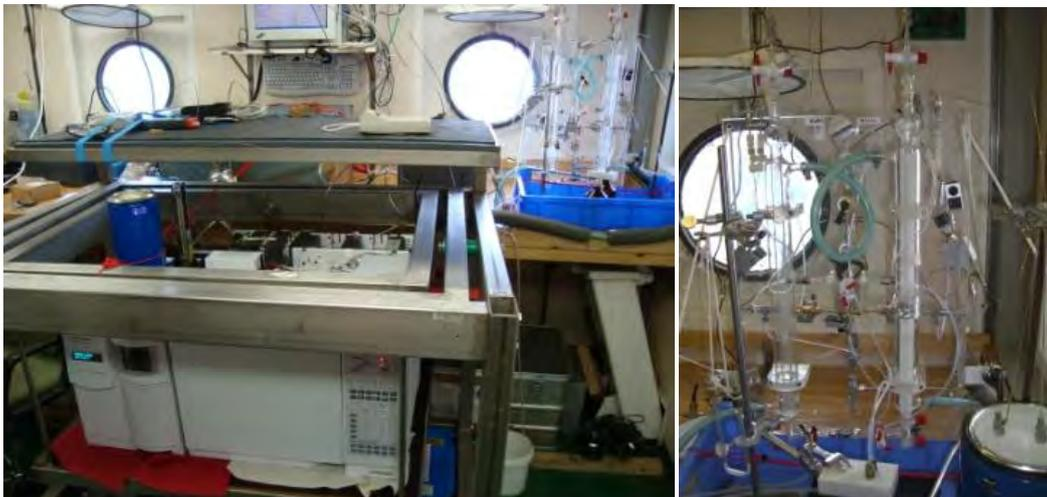
**Figure 5:** Gas chromatographic/ mass spectrometric system for the analysis of halocarbons in seawater and atmosphere.
