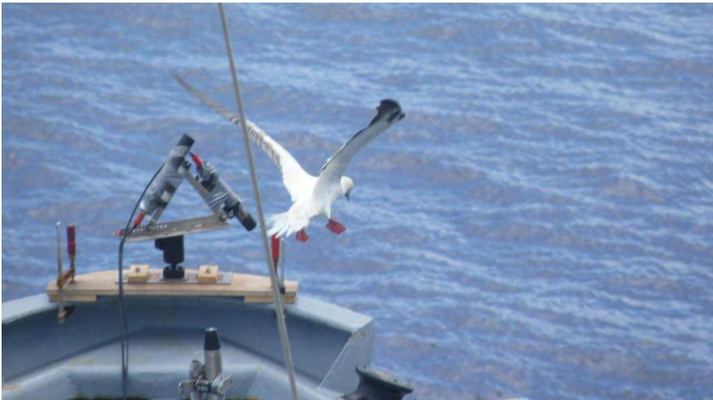
**Figure 3:** Radiometers of the Phyto-Optics group on the ships bow.
