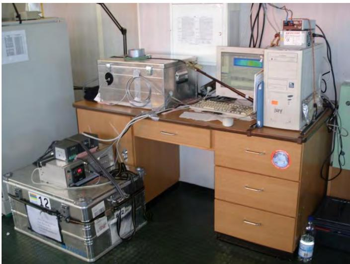
**Figure 14:** MAXDOAS setup of the iup Heidelberg. One spectrograph is used to cover the wavelength range from 327 to 470 nm.
