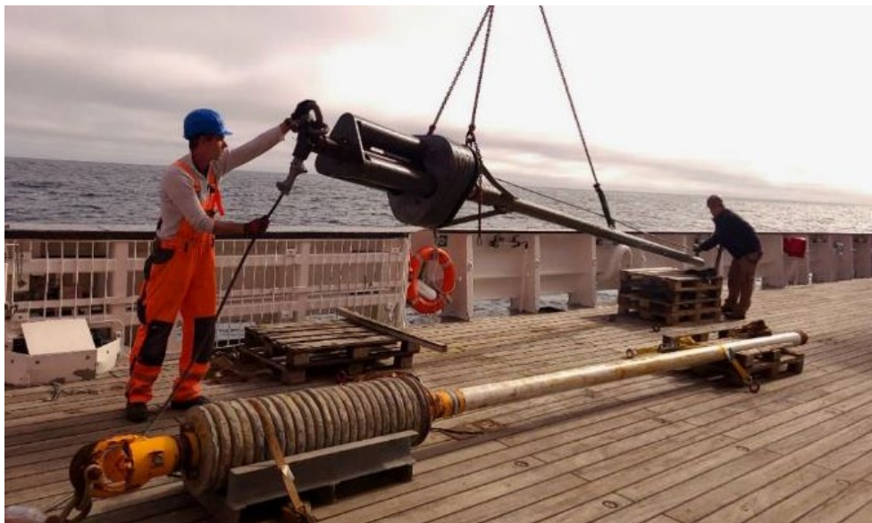
Fig. 5.7.3 Deployment of the heat-probe (Photo: Sarah-Marie Kröger, GEOMAR).
