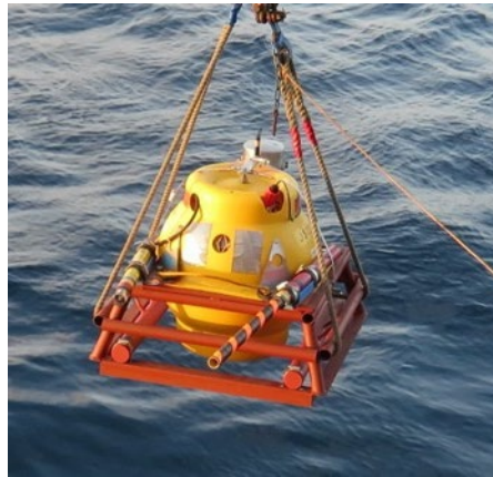
Fig. 5.2.3 Photo of JAMSTEC short-period OBS.
